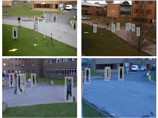
Figure 1: Typical results of the POM algorithm on PETS dataset. Each picture shows a different viewpoint at the same time frame.
