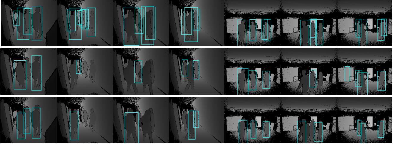
Figure 2. Situations in which we outperform state-of-the-art methods. Our approach (top) correctly detects most of the people including those that are severely occluded, whereas [15] (middle) and [13] (bottom) fail to do so.
