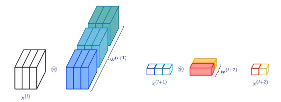
This "convolutionization" does not change anything if the input size is such that the output has a single spatial cell, however when the input is larger, it fully re-uses computation to get a prediction at multiple locations.
