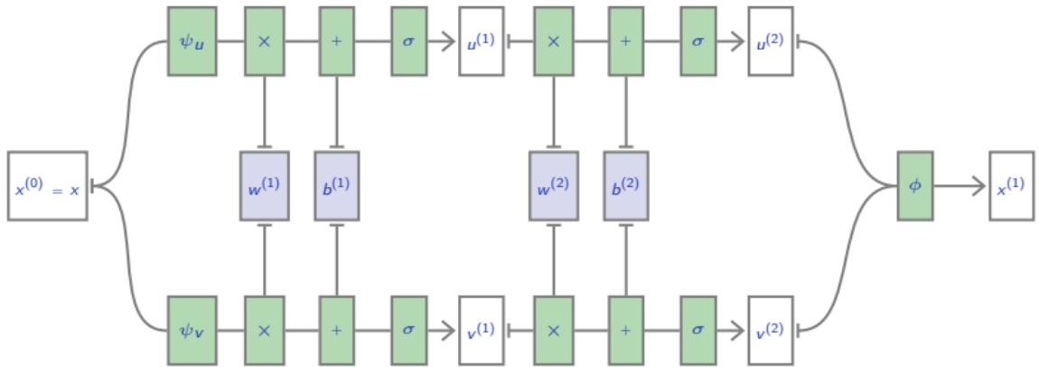
Weight sharing allows in particular to build **siamese networks** where a full sub-network is replicated several times.
