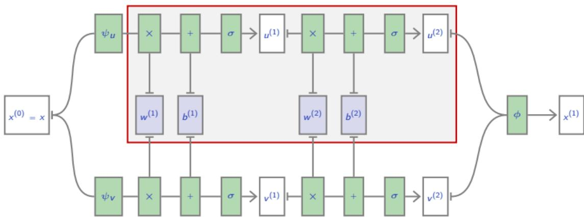
Weight sharing allows in particular to build **siamese networks** where a full sub-network is replicated several times.
