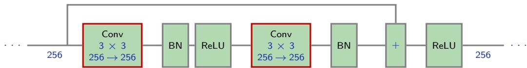
However, such a block requires  $2 \times (3 \times 3 \times 256 + 1) \times 256 \simeq 1.2m$  parameters.
