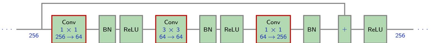
$$256 \times 64 + (3 \times 3 \times 64 + 1) \times 64 + 64 \times 256 \simeq 70k \text{ parameters.}$$
