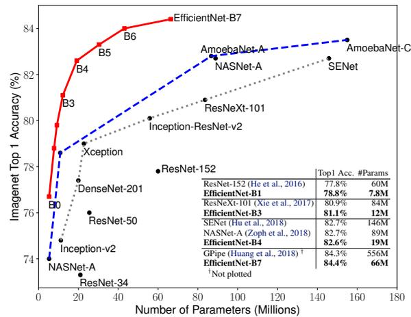
**Figure 1. Model Size vs. ImageNet Accuracy.** All numbers are for single-crop, single-model. Our EfficientNets significantly outperform other ConvNets. In particular, EfficientNet-B7 achieves new state-of-the-art 84.4% top-1 accuracy but being 8.4x smaller and 6.1x faster than GPipe. EfficientNet-B1 is 7.6x smaller and 5.7x faster than ResNet-152. Details are in Table 2 and 4.
