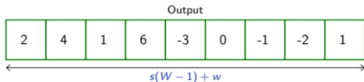
The composition of a convolution and a transposed convolution of same parameters keep the signal size [roughly] unchanged.
