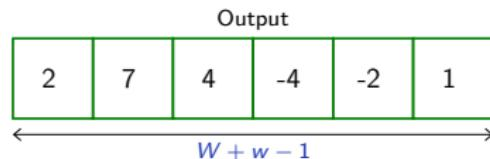
`F.conv_transpose1d` implements the operation we just described. It takes as input a batch of multi-channel samples, and produces a batch of multi-channel samples.
