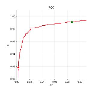
A standard measure is the area under the curve (AUC).
