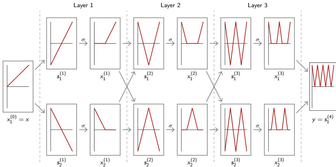
So for any  $D$ , there is a network with  $D$  hidden layers and  $2D$  hidden units which computes an  $f : [0, 1] \rightarrow [0, 1]$  of period  $1/2^D$
